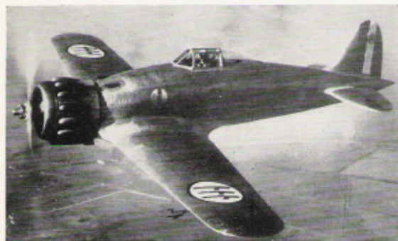
Another view of MM 336; note the perspex fairing in the rear of the cockpit.
