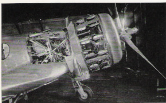
Left: Engine installation of the C.200. The characteristic "blister" on the cowling panel were necessary to accommodate the rocker-boxes of the fourteen-cylinder Fiat A.74 R.C.38 radial powerplant. Right: Experimental semi-open cockpit canopy installed on one C.200, with rear-hinging top section. The reflector-sight can also be seen in this photograph.
